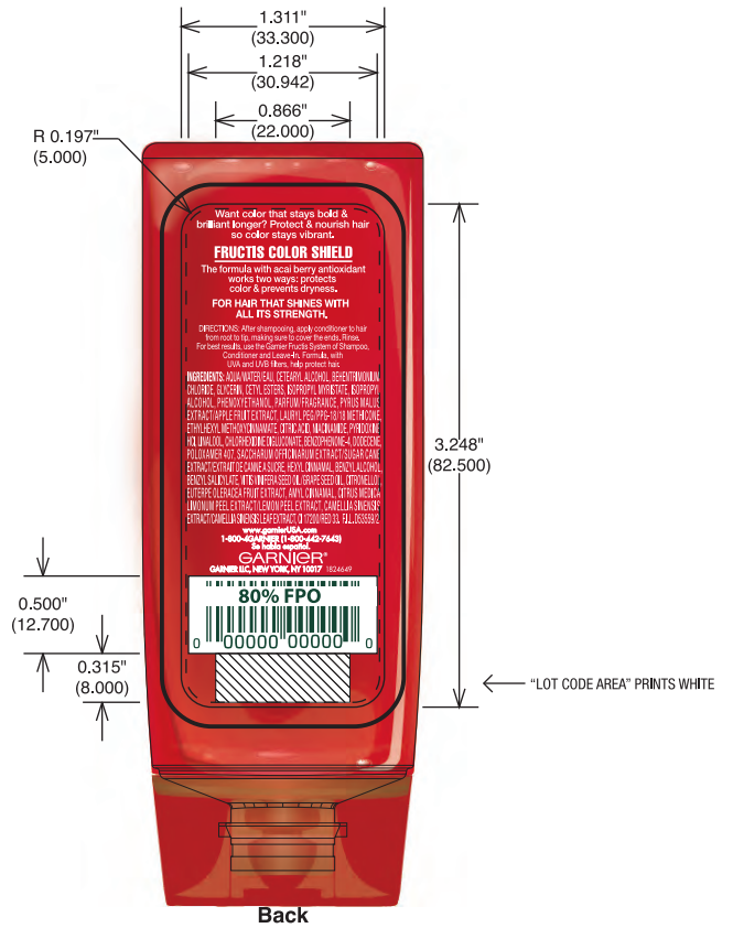
Back ALL WHITE TYPE PRINTS WHITE UPC IS FPO AND PRINTS PMS 3435 C WITH A SOLID WHITE BACKGROUND
